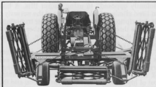
Brouwer 5 gang hydraulic lift P.T.O. mowers offer all standard Brouwer mower features plus hydraulic lift.
