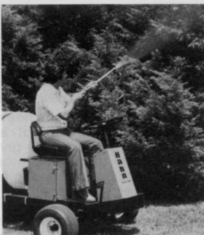
HAND GUN and 25 ft. hose permits spraying trees and shrubs on the move. Optional.
