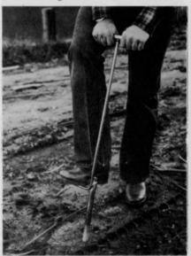
plated steel, the device is a onepiece unit with interchangeable tips for different soil types and conditions. A foot step eliminates stooping to insert the probe. Sample is removed by turning unit upside
