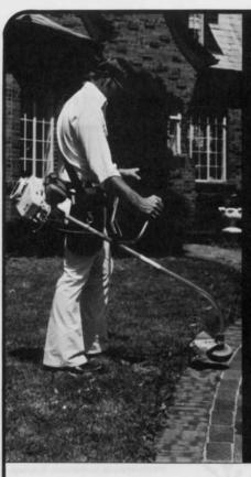
A tough 85cc engine stands behind trimming head and 2 cutting blades.
