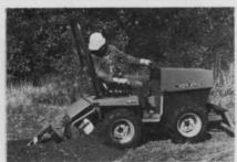
and has a 20,000 lb. test digging chain. It provides hydrostatic ground drive to all four wheels and will dig to depths of five ft. and to widths of 12-in.
