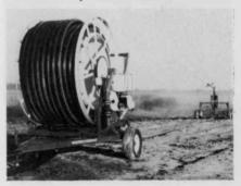
underground irrigation systems. The Nu-Way irrigation units carry up to 835 ft. of hose and are available with water turbine or gasoline engine power.
