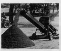
**POWERSCREENS** for preparing superfine top dressing mixes. Powered vibrating screen with elevating conveyor for direct truck-loading, stockpiling. Choice of gas or electric drive. Two models.
