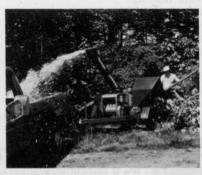
**BRUSH CHIPPERS** for high performance, low maintenance. Feature self-feeding anvil with one-piece chipping rotorflywheel-blower..."swing-away" blade access. Self-powered and PTO tractor models. Circle 112 on free information card
