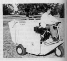
Turf Sweeper model 48 from Olathe Manufacturing, Inc., picks up clippings, leaves, rocks, cans, bottles, and other debris. It converts to a truck in minutes for year-round use. In addition to its functions with the hopper, model 48 also works as an athletic field conditioner, aerator, seeder, and top dresser. Features include 10 mph speed, hydrostatic drive, instant reel adjustment and rubber-fingered reels.
