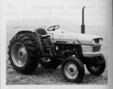
Sturdy, light utility tractors, the L345F and the L345DT from Kubota Tractor Corp. suit general contractors and city or institutional grounds maintenance. Both models have watercooled, diesel-powered engines. The L345F has four cylinders and twowheel drive and the L345DT has four cylinders and four-wheel drive.
