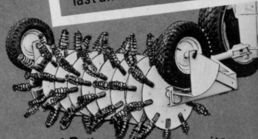
AB-1 Aeri-Boy 4 ft. swath. Simple flip-over permits quick transport.
