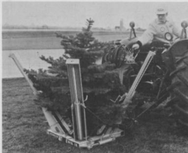
TS-20: Ball diameter, 20 in.; Ball diameter, 18 in.; Maximum tree diameter, 2 in. tree trunk (approx.) Ball weight, 109 lbs. (approx.) Tractor-mounted unit, or in combination with Vermeer T-218 Trencher.
