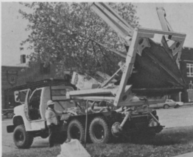
TS-66T: Ball diameter, 66 in.; ball depth, 48 in.; Maximum tree diameter, 6 in. tree trunk (approx.) Ball weight, 3168 lbs. (approx.) Available as a truck-mounted unit only.
