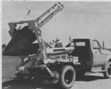
NEW! TS-44M . . . far greater maneuverability than ever before. No more guesswork. The TS-44M hydraulically extends (up to 21 in.) and shifts (up to 15½ in. left and right of center). It's fast, accurate. Cuts set-up time to a fraction.
