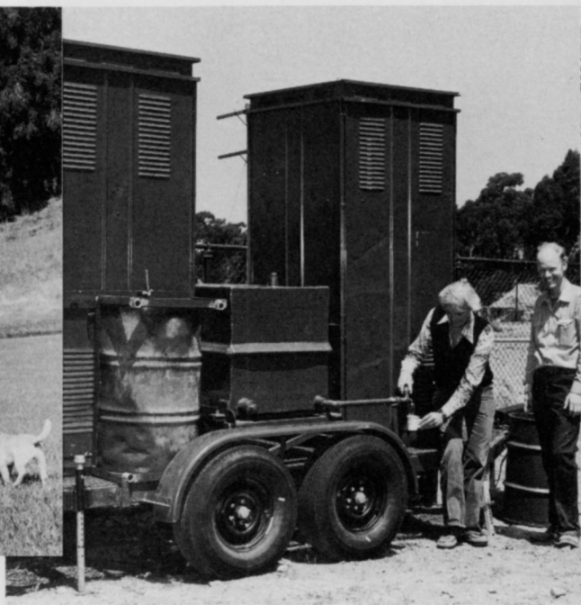
Special toilet trailers for back country campouts eliminate road damage by heavy pumpout trucks servicing out of the way latrines. The trailer carries water, barbecue pits, garbage cans, and two chemical toilets.
