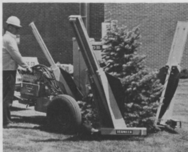
TS-30: Ball diameter, 30 in.; Ball depth, 26 in.; Maximum tree diameter, 3 in. tree trunk (approx.) Ball weight, 355 lbs. (approx.) Trailer or tractor-mounted units. Flat-bottom tree spade option.
