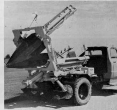
NEW! TS-44M . . . far greater maneuverability than ever before. No more guesswork. The TS-44M hydraulically extends (up to 21 in.) and shifts (up to 15½ in. left and right of center). It's fast, accurate. Cuts set-up time.
