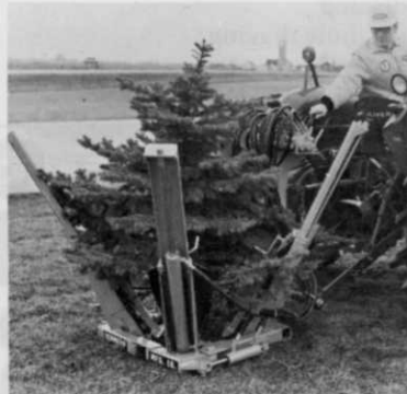
TS-20: Ball diameter, 20 in.; Ball diameter, 18 in.; Maximum tree diameter, 2 in. tree trunk (approx.) Ball weight, 109 lbs. (approx.) Tractor-mounted unit, or in combination with Vermeer T-218 Trencher.
