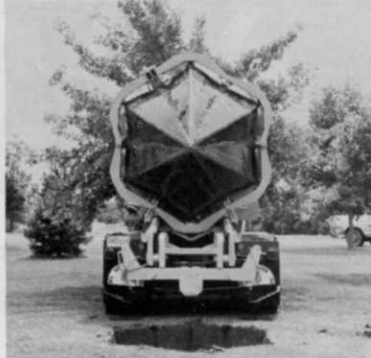
TS-84: Ball diameter, 84 in.; Ball depth, 54 in.; Maximum tree diameter, 8 in. tree trunk (approx.) Ball weight, 8,000 lbs. (approx.) Available as a truck-mounted unit only.
