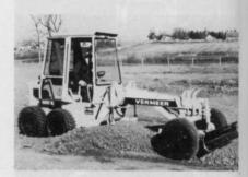
The four-wheel drive grader is powered by a 28-horsepower, air cooled, Deutz diesel engine with hydrostatic drive and all-hydraulic control. It is also equipped with a six foot, front-end dozer blade which cuts to a maximum of four inches below and 12 inches above grade. The eight foot center blade cuts three inches below and ten inches above grade.
