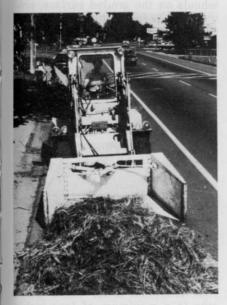
The "Claw," from Wastequip, Inc., is used to pick up tree prunings, leaves, grass, and other yard and garden refuse normally placed along gutter lines of municipal streets. The machine works equally as well with wet and dry materials.
