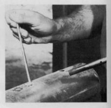
Uni-Al, a low temperature brazing rod, makes it possible to repair aluminum "items such as irrigation pipes, lawn mower housings, and
