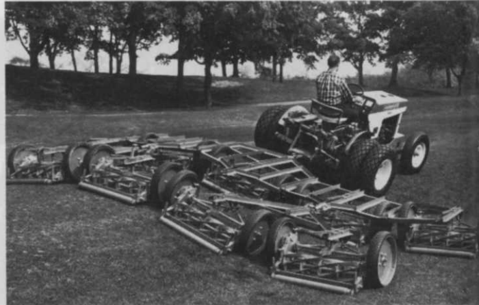
There are forty-five blades to sharpen on this gang mower, a true maintenance challenge.
