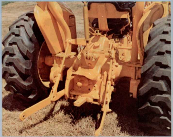
Leveling 3-point-mounted tools is easy using the hand cranks located on the lift link and right draft link.
