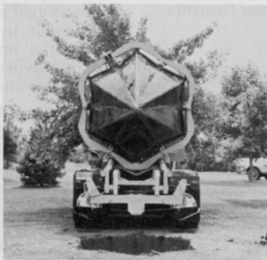
TS-84: Ball diameter, 84 in.; Ball depth, 54 in.; Maximum tree diameter, 8 in. tree trunk (approx.) Ball weight, 8,000 lbs. (approx.) Available as a truck-mounted unit only.
