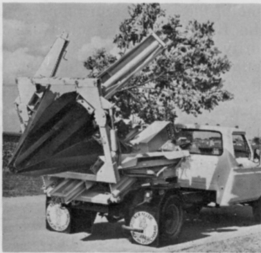
TS-44T: Ball diameter, 44 in.; Ball depth, 40 in.; Maximum tree diameter, 4 in. tree trunk (approx.) Ball weight, 1173 lbs. (approx.) Available as truck-mounted trailer-mounted or Vermeer M-485 tractor mounted unit.
