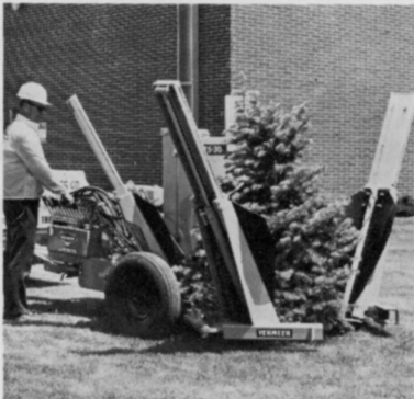
TS-30: Ball diameter, 30 in.; Ball depth, 26 in.; Maximum tree diameter, 3 in. tree trunk (approx.) Ball weight, 355 lbs. (approx.) Trailer or tractor-mounted units. Flat-bottom tree spade option.
