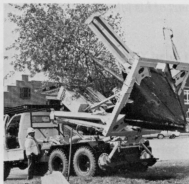
TS-66T: Ball diameter, 66 in.; ball depth, 48 in.; Maximum tree diameter, 6 in. tree trunk (approx.) Ball weight, 3168 lbs. (approx.) Available as a truck-mounted unit only.
