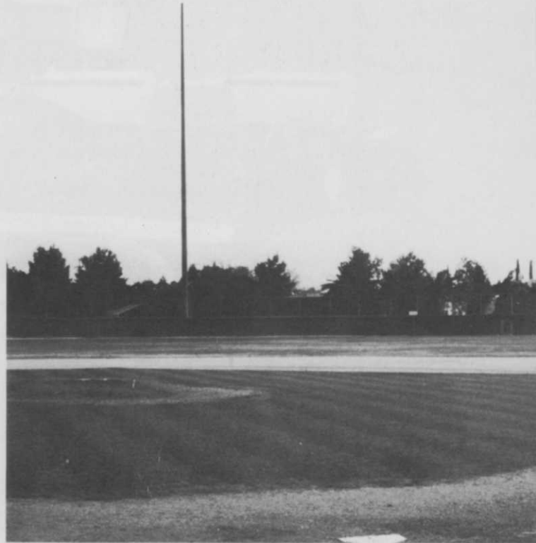
University of Arizona field has skinned areas of a sandy soil composition. Turf is common bermuda, overseeded with annual ryegrass for winter play.
