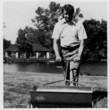
models hold from 65 to 78 lbs. of material. The spreaders have a slide shutoff activated by a handle crank and a cam gauge adjusted opening for accurate application of granular fertilizer, pesticides, seeds and more.
