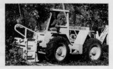
cluding a trencher, backhoe or tamper to perform such tasks as composting, snow removal, brush raking, and trenching and backfilling. A winch can be added. The tractor features hydrostatic drive, logging tires, coordinated or front steering,
