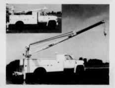
boom are operated by a 20-ft. pendant remote control. The manually extendable booms can lift up to 3 tons powered by battery or by AC with stationary mounts.
