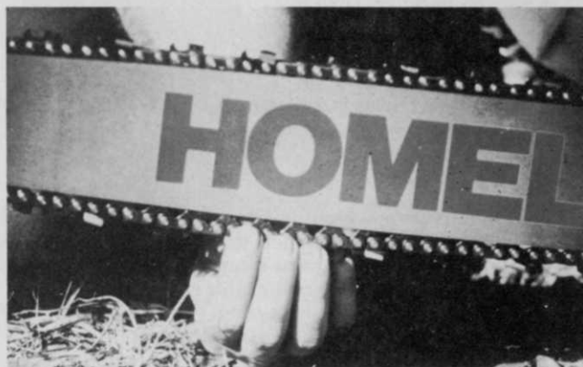
Bucking bar (top) adds leverage to cutting. You should not be able to see the drive links on the underside of the cutting bar with the chain in the rest position if the chain has proper tension. (above, lower)
