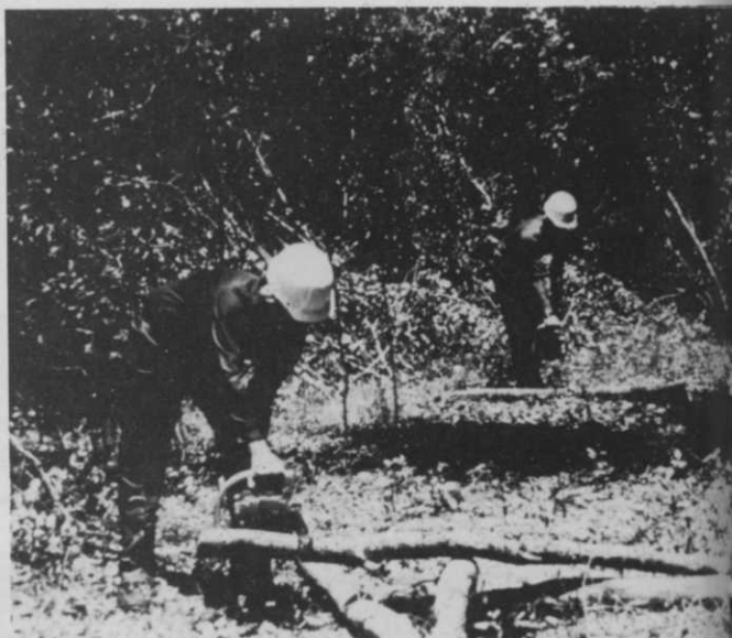
When two men are using chain saws at the same time, they should be at least ten feet apart and aware of each other's movements.
