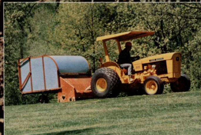
Adjustable sway blocks and 3-point lift links handle Category 1 or 2 tools.
