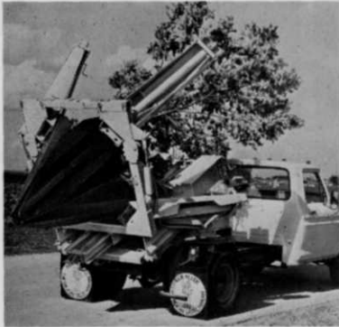
TS-44: Ball diameter, 44 in.; Ball depth, 40 in.; Maximum tree diameter; 4 in. tree trunk (approx.) Ball weight, 1173 lbs. (approx.) Available as truck-mounted trailer-mounted or Vermeer M-485 tractor mounted unit.
