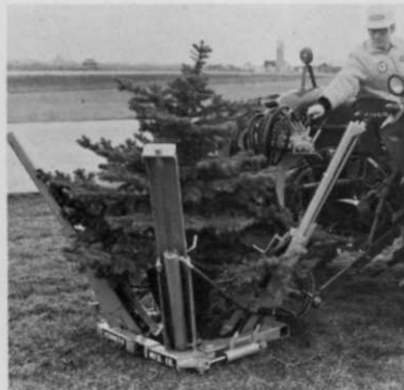
TS-20: Ball diameter, 20 in.; Ball diameter, 18 in.; Maximum tree diameter, 2 in. tree trunk (approx.) Ball weight, 109 lbs. (approx.) Tractor-mounted unit, or in combination with Vermeer F-218 Trencher.
