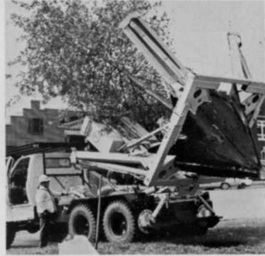
TS-66: Ball diameter, 66 in.; ball depth, 48 in.; Maximum tree diameter, 6 in. tree trunk (approx.) Ball weight, 3168 lbs. (approx.) Available as a truck-mounted unit only.
