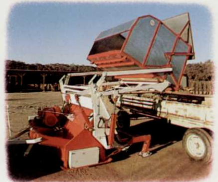
Hydraulic dumping feature of HL models can dump at any height up to 8½'.
