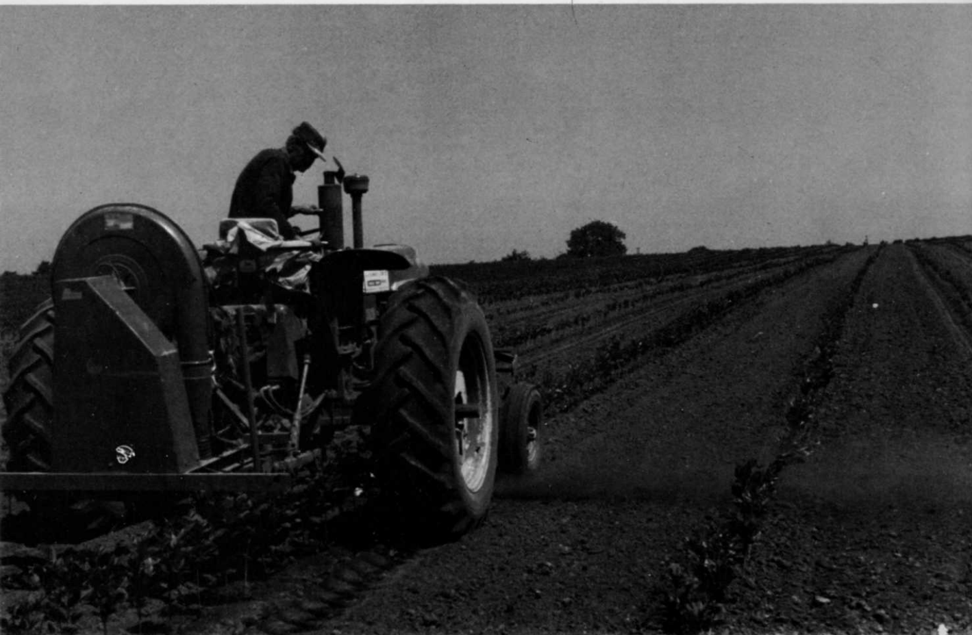
A specialized blower used to weed between the trees and to remove soil build-up around the stems of the seedlings in preparation for the budders.
