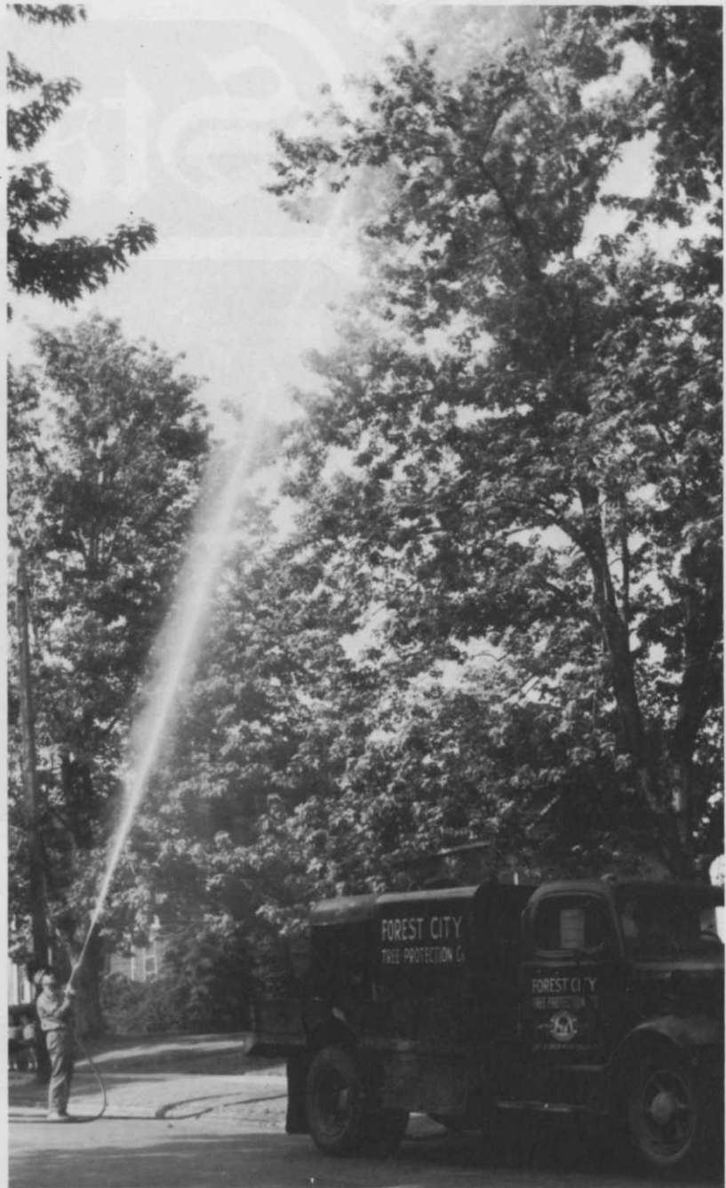
A high pressure hydraulic spray rig can cover the taller trees.
