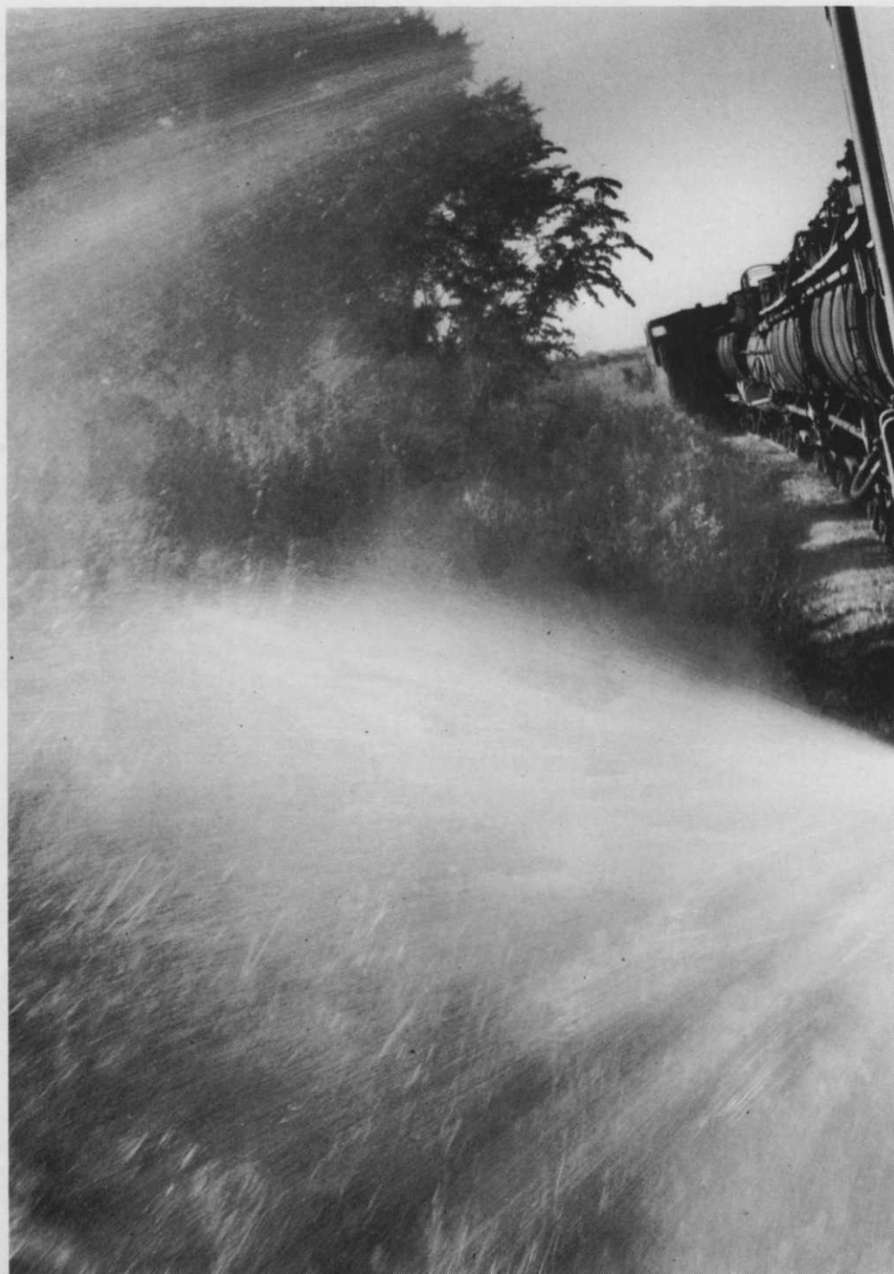
A long stretch of railroad rights-of-way can be sprayed utilizing a railroad spray car and a train of tankers.
