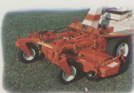
Front wheels support cutter deck for super stability.
