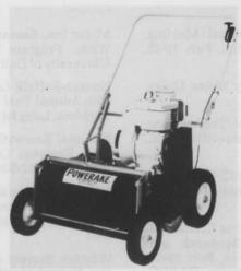
POWERAKE by F.D. Kees offers new features to safe time and energy. The Model 100528 boasts a centrifugal clutch for easier starting and operator safety, a single-action height adjustment, dual filter air cleaner, and an improved heavy-duty wheel with grease fittings. The Powerake utilizes a 5 h.p. Briggs & Stratton engine, and 28 hardened-steel, self-cleaning fingers to clean a 20-in. swath. The raking assembly is interchangeable with the aerator assembly of the Kees Powerslice.
