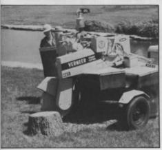
Vermeer Stump Cutters. Fastest, easiest, most economical method of removing tree stumps. With four powerful machines, each equipped with a big hydraulically controlled cutting wheel that actually chews even large stumps to chips 6-24 in. below the surface... in minutes!
