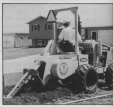
Vermeer Trenchers. Multi-purpose underground machines with a wide variety of money-saving dirt-handling attachments. On tracks or rubber tires. With power ranges from 18 to 195 hp. With digging capacities of 4-36 in. wide, down to 12 ft. deep. Vermeer Vibratory Plows, for installing cable directly underground without damaging finished surfaces or landscapes.
