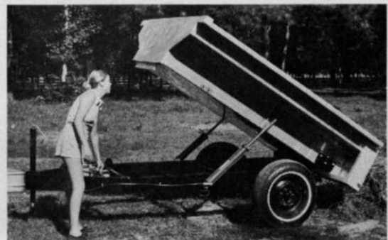
HYDRA DUMP TRAILER Aluminum Hydraulic Dump Bed
