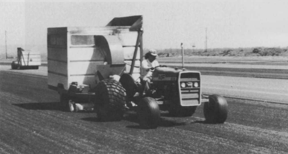
Vacuums clean up after mowing. A land plane is used to smooth the surface for seeding.
