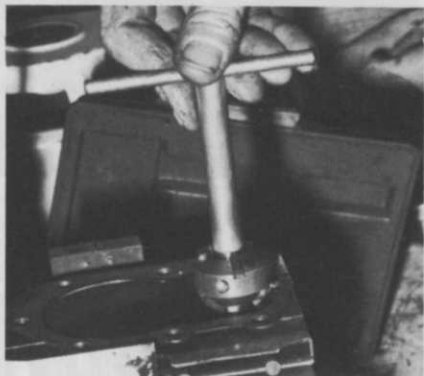
Then the cutter handle. Rotate this unit until the seat is smooth.
