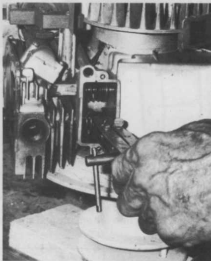
Insert the valve spring compressor over the spring and valve retainer clip. Tighten the tool to compress the spring and tilt it to remove the clip from the end of the valve.
