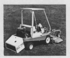
Jacobsen has made available a water cooled engine as an option for the 72-inch Out Front Commercial riding rotary mower. The heavy duty engine option was added for users who require longer than usual operating intervals between engine maintenance. It has a comparatively low operation temperature (180°F) which extends the life of valves, rings and other internal working parts, a characteristic of water cooled power.
