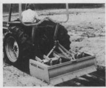
A new 20-cubic-foot capacity rear-mounted box scraper which fits standard category II 3-point quick-coupler hitches has been introduced by the Woods Division of the Hesston Corp. It weighs 750 pounds and is designed for tractors with maximum 60 hp or 6,000 pounds gross weight.
