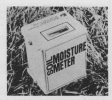
A battery-operated electronic Soil Moisture Meter which measures and displays the amount of moisture in the soil instantly, has been introduced by Agtronics Manufacturing. The probe measures conductance in the soil.
