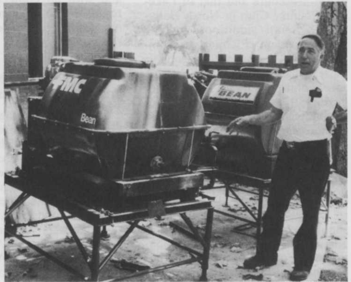
Superintendent Lokey displays spray tanks adapted for use on Cushman scooter and mounted on jacks for easy loading.
