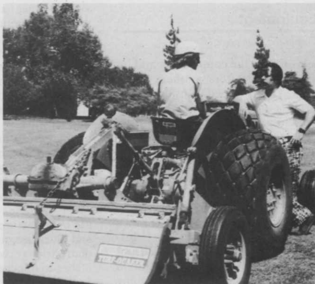
Howard Turf-Quaker aerifies turf at Lakeside Country Club. Equipment consists of tractor-towed rototiller with slicing reel.
