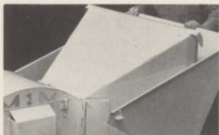
Feed chute folds to enclose the cutter chamber during storage or transportation. It is side hinged so it may be swung away for easy access to cutter chamber.
