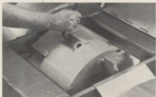
Double-edged knives staggered around the large 16-in. diameter solid steel rotor provide smooth, efficient cutting without an external flywheel. Easily accessible.
