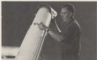
Telescoping discharge chute rotates to give maximum flexibility to fill dump boxes. An adjustable bonnet at end of the chute controls direction of discharge.
