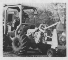
A new, high-production machine, designed for direct burial of underground distribution systems, has recently been introduced by Vermeer Manufacturing Co.
