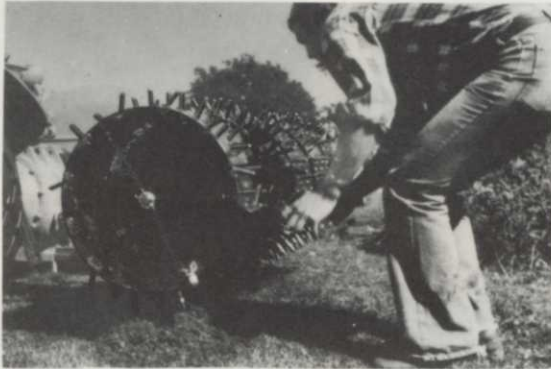
TCA-601 Supreme with conversion unit — 180 tines (300 if necessary). Has hinged door and removable sides. Collects plugs internally or can be used same as standard model.
