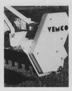
Vemco Flail Mowers is expanding marketing of flail mowers for use on tractors up to 35 hp, with a category "O" or category "I" three point hitch and a rear P.T.O. shaft. They are available in cutting widths of 42", '48", and 60", and are capable
