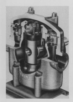
HYPRO, a division of Lear Seigler Inc., announces a new twin-piston pump. The unit, called the Series 5900 Super-Twin, is designed to operate at working pressures to 500 PSI. at 600 RPM (the maximum speed). At 500 PSI, the unit pumps 18.5 GPM. The manufacturer recommends chain coupling drive with in-line shafts. The pump can also be belt driven.
