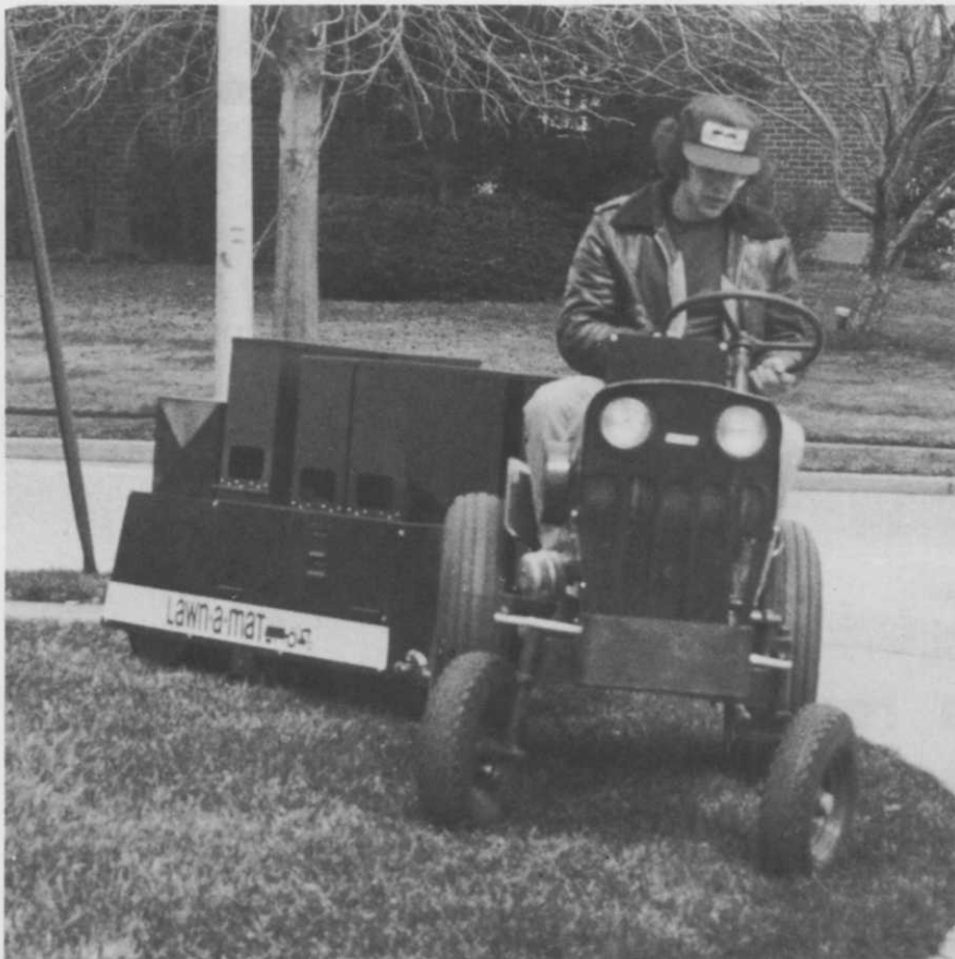
Above, the all-purpose combine can cover irregular properties with relative ease and can be backed into corners when necessary. Below, the rig is transported to the job site by a trailer then backed off in a matter of seconds.
