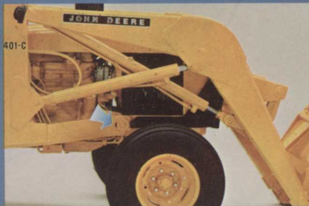
Loader booms are reinforced at the arch point with the plate applied to both sides of the boom. Slotted mounting point (arrow) permits horizontal float.
