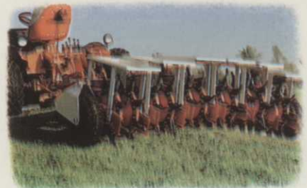
Notice how each section rides close to uneven contours of ground to provide even aeration. Individual weight trays provide pressure.
