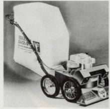
Billy Goat introduces the KD-50SP model suction sweeper with free wheeling in neutral and a "deadman" clutch for added safety. Self-propelled chains provide power takeoff from engine to axle, adjustable height levels for various terrain, handlebar controls. The KD-50SP is powered by a 187 CC's Briggs and Stratton gas powered engine.
