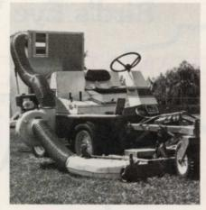
A new turf vacuum that uses an independent power source is now available from Jacobsen as an attachment to their Out Front Commercial riding rotary mower. The "Turf Vac" has a 1-cu. yard hopper that attaches to the back of the Out Front Commercial and a 7 hp Kohler engine that attaches to the machine's right side. Power is ample for picking up small debris as well as clippings and leaves. Noncorrosive materials are used wherever moisture might be a problem.
