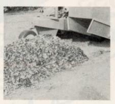
Hustler's new Catcher/Compactor simplifies disposal of grass clippings and lawn debris without the use of auxiliary power or noisy blowers. It relies on tractor drive wheels for paddle conveyor power.
