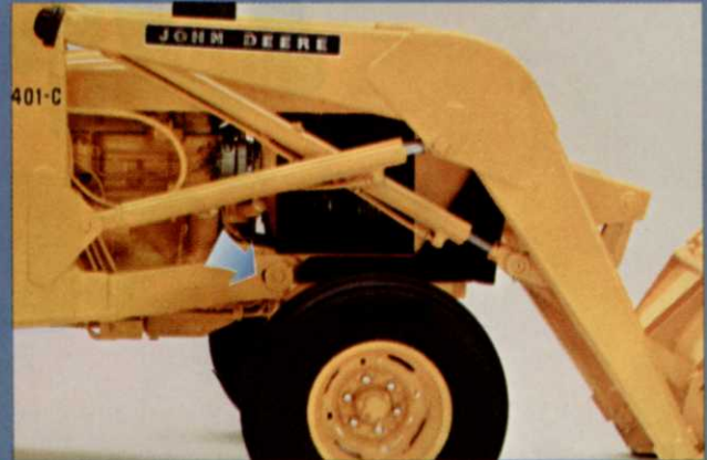
Loader booms are reinforced at the arch point with the plate applied to both sides of the boom. Slotted mounting point (arrow) permits horizontal float.
