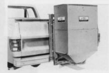
Western's Super Spreader features an adjustable mounting height for on-the-job flexibility. A low height setting allows the salt to get directly under parked vehicles, while a high setting gives one-pass coverage with a maximum spread width.
