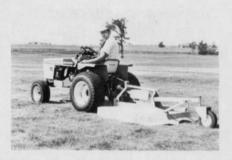
Two models of rear mounted rotary mowers for cutting grass and light brush have been approved by the Simplicity Manufacturing Co. for application with its 19 ½ hp 9000 Series garden tractor. The equipment comes in 48 in. and 60 in. widths. All are attached by Category O three-point hitches for quick hook-up.
