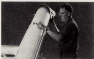
Telescoping discharge chute rotates to give maximum flexibility to fill dump boxes. An adjustable bonnet at end of the chute controls direction of discharge.
