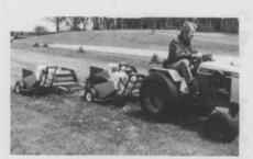
The Three Gang Mower has been added to the Lawn Genie line by Mathews Company. It mows, mulches, thatches and shreds up to 37 acres per day at 3 m.p.h. and 49 acres per day at 4 m.p.h. Like the 3 ft. Lawn Genie, the new machine features adjustable cutting heights and a drawbar for quick, easy attachment or removal from the hitch. The free swinging, reversible blades are easily removable for sharpening or reversing.
