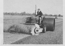
The Sweepster Model HF from Sweepster, Inc., offers a fast, effective way to remove grass clippings and thatch for faster, healthier turf growth. It has a six foot wide brush with gentle yet durable polypropylene bristles. Mounted on an industrialsized tractor, it sweeps a five and one-half foot path and quickly windrows grass clippings. Spring tension allows the HF to follow ground contours and prevents the brush from digging in and scalping the sod.
