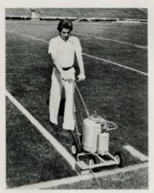
A new TrueLine pressure spraytype striper developed by Trusco Mfg. Co. uses CO, pressure and has a 7-gal, paint tank for striping large parking areas, traffic lanes, and all athletic fields. The paint and pressure tanks are mounted on welded chassis that ride on four ball bearing wheels.
