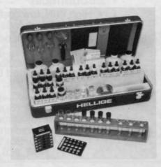
The new Model 697-A Soil Tester by Hellige provides quick, accurate tests and soil treatment instructions for the 14 most important chemical soil elements. The scientific test methods were devised by Prof. E. Truog, chairman, dept. of soils, University of Wisconsin.
