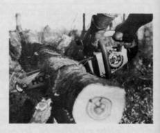
Homelite has introduced a gasoline-powered chain saw model with triaxial anti-vibration system, deluxe safety hand guard and single trigger with safety-interlock.
