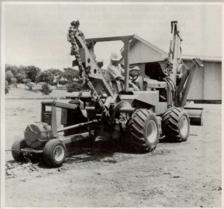
The COMBO on R65 Modularmatic vehicle. A COMBO-equipped vehicle's work capability can be extended even more with a utility backhoe (pictured) and hydraulic boring unit. Backfill blade is standard.
