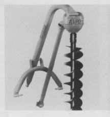
Five Star Engineering has developed a heavy-duty industrial auger digger. The Five Star Digger is sold under a three year warranty and fits all tractors with Cat. 1 & 11 3-pt. hitches. Bevel gear is machined and hardened and Woodruff keyed to the output shaft with a reduction of 3.18 to 1. Pinion is one piece with splined input shaft, machined, hardened and straddle mounted between two tapered roller bearings.
