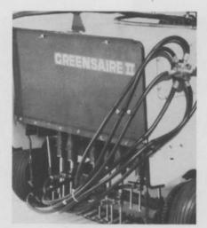
A new liquid injector attachment capable of injecting nematicides up to three inches deep through small, hollow tines, will be introduced this spring by Ryan. The new attachment is powered by Ryan's Greensaire 11 aerator and connects to any pressurized (150-400 psi) spray tank. The attachment can be installed in approximately 30 minutes. The new attachment can treat up to 8,000 sq. ft. per hour.
