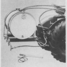
A new 30 gallon sprayer for Economy Power King and Jim Dandy model tractors will handle liquids, water-soluble chemicals or wettable powders. The sprayer can be used for fertilizer applications or for spraying insects, weeds, trees or bushes. The unit is equipped with a 100 lb. pump, a pressure gauge, suction strainer, shut-off and relief valves, a tree spray nozzle and a spray boom with four nozzles that can be mounted on front or rear of the tractor.
