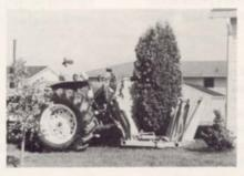
down 26" while a large gravity-feed water tank bathes the operation in water for better digging. The unit mounts easily to a standard category II 3-point hitch on a 3 plow and 5 gpm hydraulic pump capacity.
