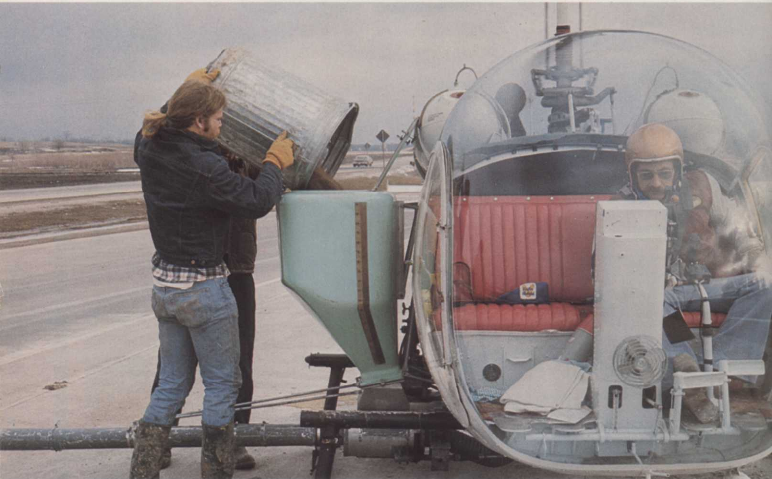
Above: special aerial bucket carries enough seed for eight acres. Right: an altitude of 45 feet with a speed of 45 miles per hour yields a swath width of 45 feet.
