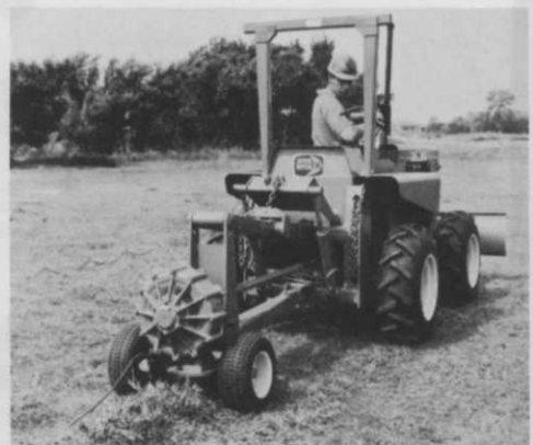
Vibratory plow modules are available for Modularmatic vehicles in the 30-HP to 65-HP range.
