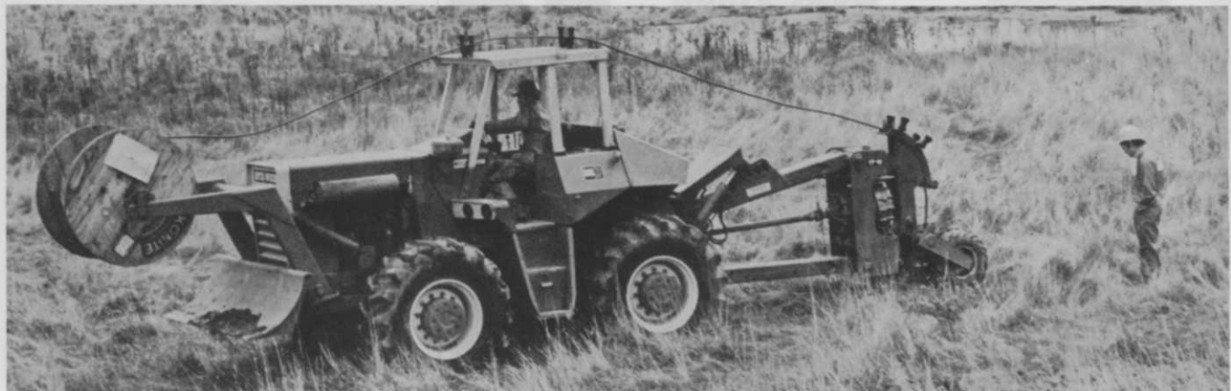
The 10-ton R20 is the only vibratory plow equipment in its class designed exclusively for underground work.
