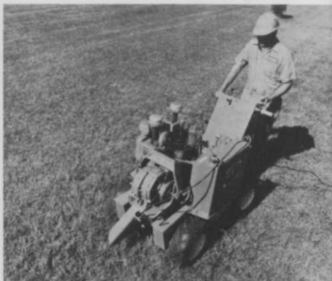
The 25-HP VP12 service plow is compact to work in restricted areas. Positioning of controls provide easy operation.
