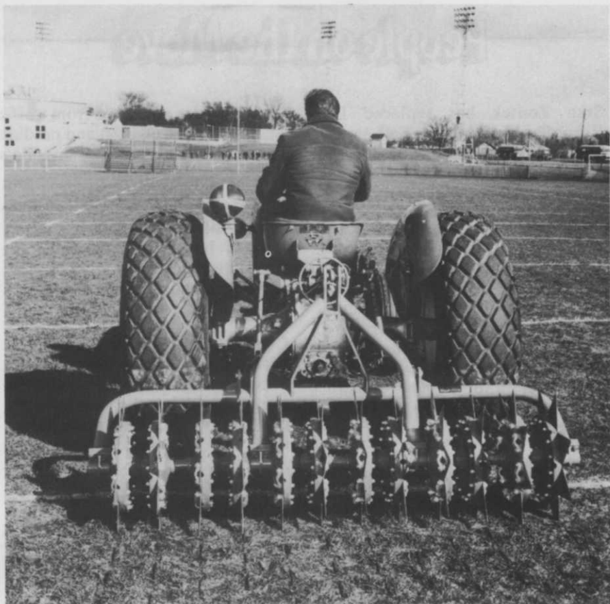
An athletic field normally can be aerified in one-half day with automatic equipment pulled by a tractor. It restores a soft springiness to previously compacted ground by removing soil cores so air, water and fertilizer can penetrate the rootzones.
