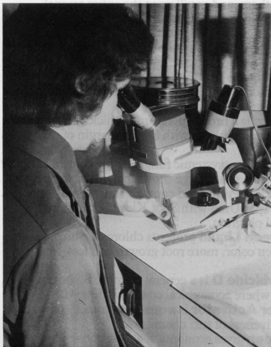
Kevin Kern, technician, uses vibrator developed by Seed Technology, Inc., to check turfgrass seed sample. Vibrator directs seed past operator at a variable speed rate depending on type and condition of seed. Magnification range is 1\frac{1}{2} to 25 power. Unit permits careful examination of seed at a rate 10 times faster than hand method, which also includes use of a hand lens.
