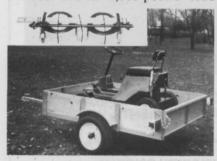
capacity. Its tilting bed and hinged tailgate — which doubles as a loading ramp — makes it easy to manipulate which doubles as a loading ramp — makes it easy to manipulate cargo that could not be handled any other way.
