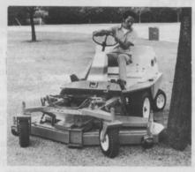
up around trees and plantings, as well as cutting under shrubs and overhanging branches. Its twowheeled cutter deck carrier is articulated for mowing gullies, slopes and knolls. Four caster wheels and three rollers on the deck prevent scalping. During transport, the unit can climb curbs with no damage to deck components.
