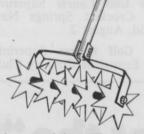
without weights. The unit will not lift turf and the company said it is faster and more efficient than a rake in cultivating and loosening smaller compacted areas where large equipment is not suitable.
