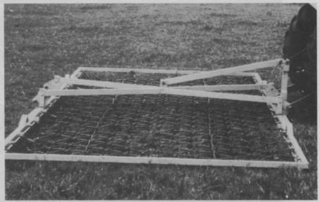
FLEXIBLE: Fuerst Brothers, Inc., says this new 3-point mounted frame fits either their Hercules or Peerless model harrows. It is also said to permit operation at higher speeds, provide better control and increase ease of transport. The harrow is attached to the frame so that full flexibility is retained and frame cannot ride on the ground. Circle 701 on free information card.
