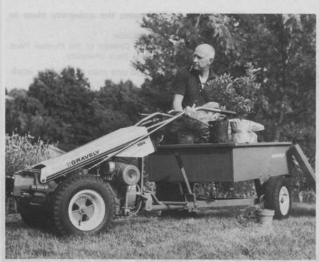
TRACTOR: This is Gravely's new Model 524, 8 HP, 4-speed, manual start tractor. The unit is powered by a Kohler K181, air cooled engine. The engine is designed to operate efficiently under all conditions and to deliver full-rated horsepower. All models feature Gravely all-gear and steel shaft drive from the engine to the attachment. Circle 710 on free information card.
