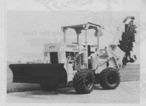
TRENCHER: Vermeer Manufacturing Co. has a new heavy-duty, rubber-tired trencher. According to the company, the M-475 offers a choice of two engines — both liquid-cooled power in the 192 Ford gas or 254 Ford diesel engine. The unit retains all of the heavy-duty construction and handling features of the M-470, including 15,000 lb. capacity, full floating Rockwell axles, hydraulic four-wheel brakes, power articulated steering and a heavy-duty electrically welded frame, says the manufacturer.
