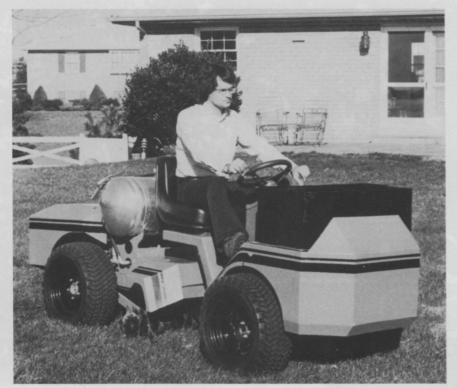
UNI-TRAK: Here's a unit for the automated lawn industry that features a 20 gallon tank sprayer with a flood jet nozzle. Uni-Trak Equipment Co. also says that the machine's four hoppers can hold up to 60 lbs. of granular material or seed. The unit is powered by an 16 HP Onan gasoline engine.
