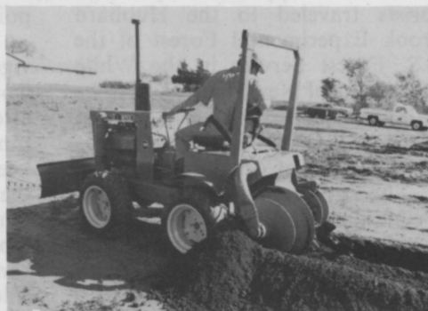
30-HP Model V30 — Trenching capabilities to 18" width, to 6' depth
