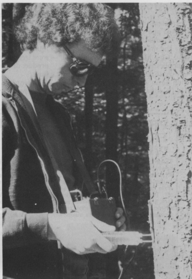
One of the newer and probably best use of the Shigometer to the professional arborist is the way in which the cambium can be quickly metered and checked for vigor as Al Butler demonstrates.
